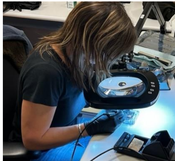
Mindy Leffel soldering wires to PMT divider base connector
